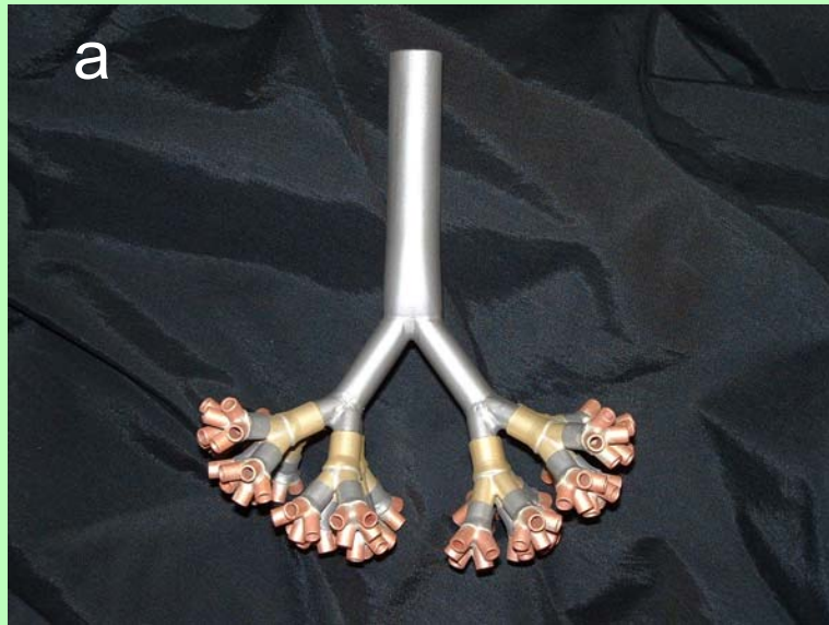
Keitch model lung: (a) branching of the bronchial tree, (b) the complete set-up
